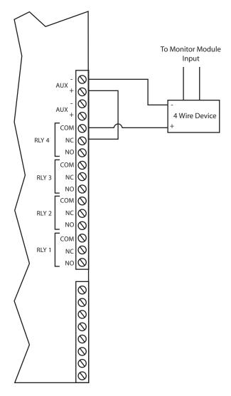
Figure 1: Four Wire Device Wiring (Typical)
