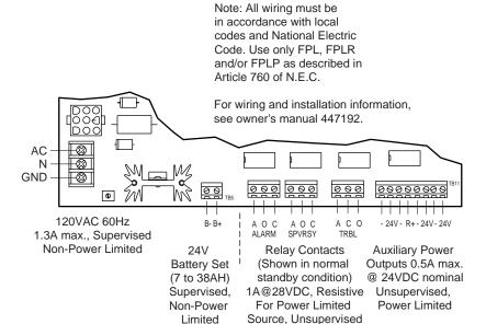
Addressable Device Circuit Style 4, 6 or 7 Operation (set jumper P1 for proper style) 24VDC nominal Wire Resistance-20 ohms/line Supervised, Power Limited See Owner's Manual for Compatible Devices
